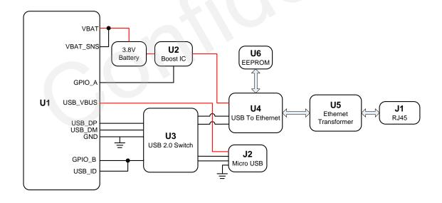
Figure 1: Hardware Design Diagram of Converting USB 2.0 to 10/100M Ethernet
