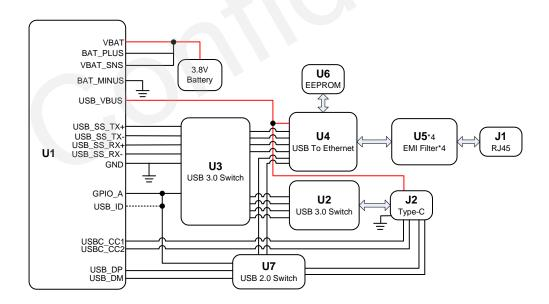
Figure 2: Hardware Design Diagram of Converting USB 3.0 to 10/100/1000M Ethernet
