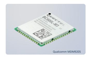
BC600L-M3 is a multi-mode LTE Cat M1/Cat NB2/EGPRS module with integrated GNSS functionality. It is fully compliant with 3GPP Rel. 14 specification and offers a maximum data rate of 589Kbps downlink and 1.12Mbps uplink. It features ultra-low power consumption by leveraging the integrated RAM/flash as well as the ARM Cortex A7 processor supporting ThreadX, achieving up to 70% reduction in PSM leakage and 85% reduction in eDRX current consumption compared to its predecessor.
