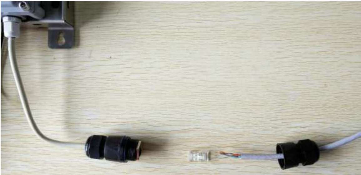
(1) Unscrew the RJ45 water proof joint
