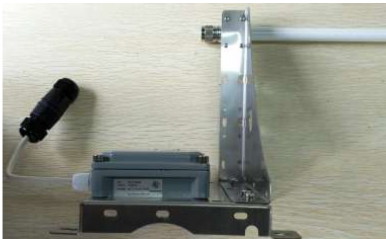
(1) LoRaWAN antenna fixture position
