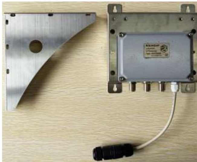
Figure 3-4 Fix the GW to the main fixture
