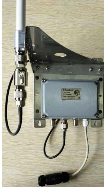
Figure 3-5 Fix antenna to the fixture
