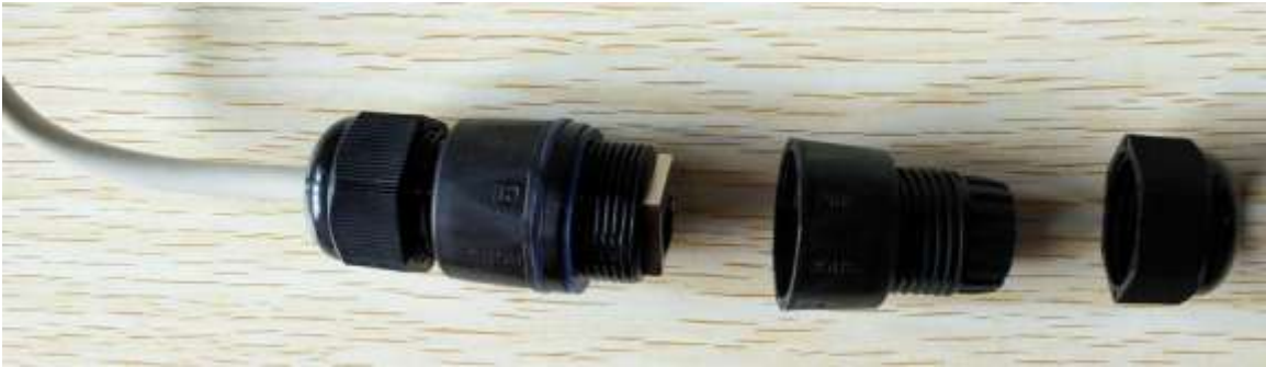
(1) Unscrew the RJ45 water proof joint
