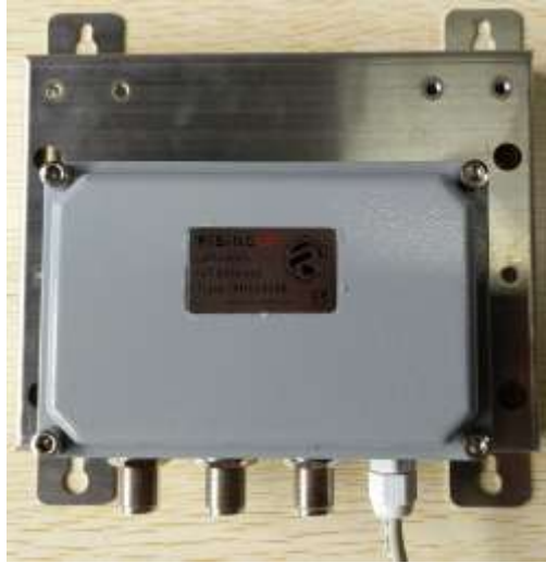
Figure 3-4 Fix the GW to the main fixture
