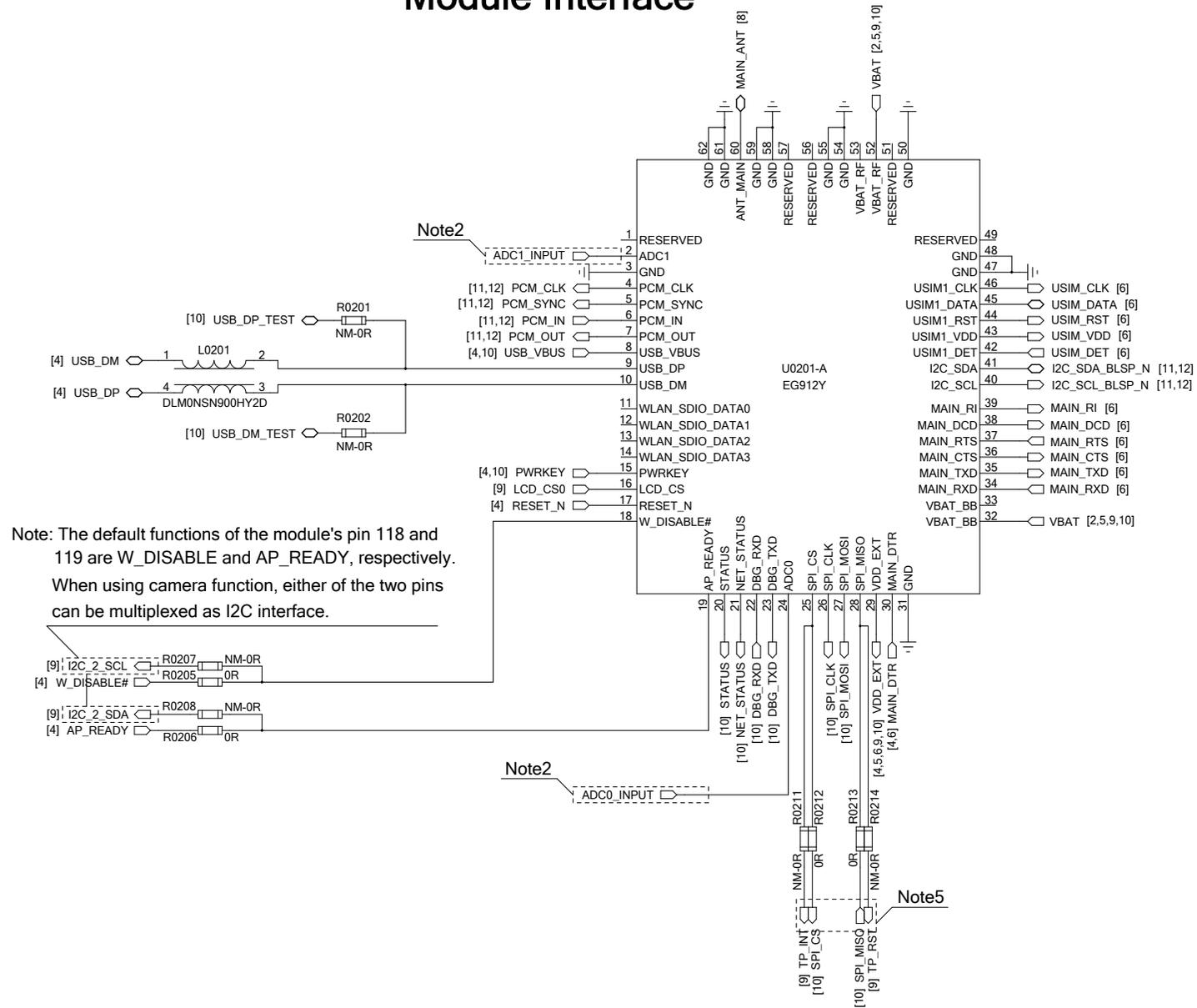
Note: The default functions of the module's pin 118 and 119 are W\_DISABLE and AP\_READY, respectively. When using camera function, either of the two pins can be multiplexed as I2C interface.
