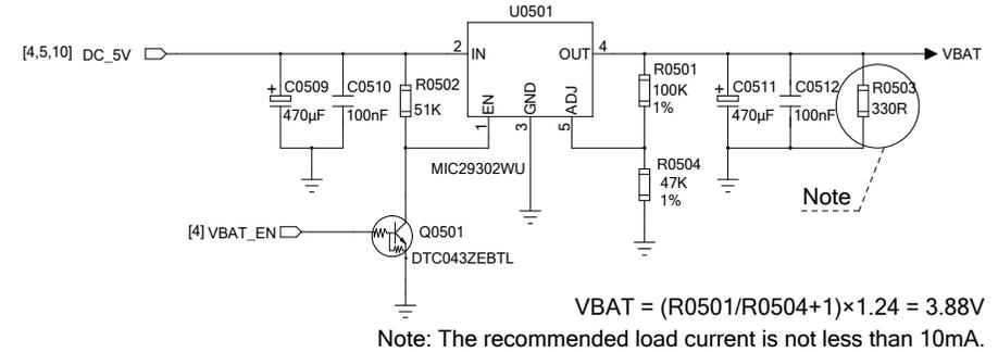
$V_{BAT} = (R0501/R0504+1) \times 1.24 = 3.88V$
