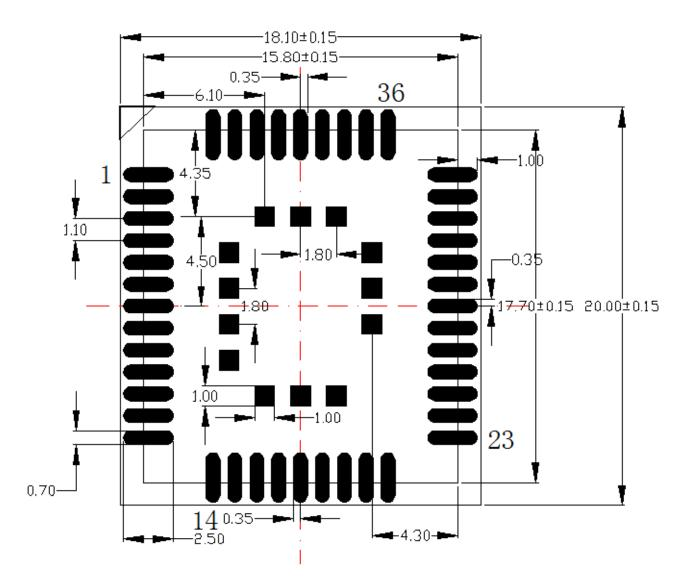
Figure 15: Recommended Stencil Design for BC66/BC68 (Unit: mm)
