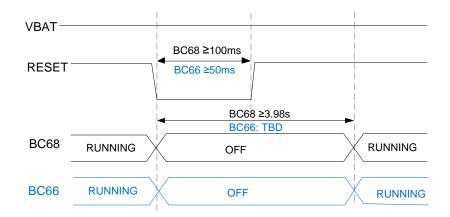
Figure 8: Timing of Resetting Module
