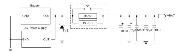
Figure 3: Reference Circuit of Power Supply
