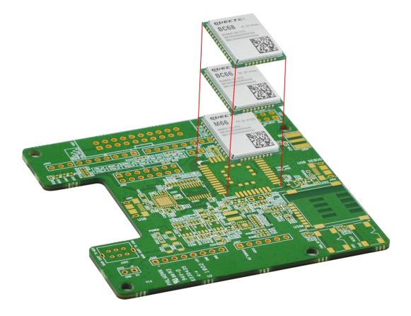
Figure 17: Installation Sketch Map for BC66/BC68/M66
