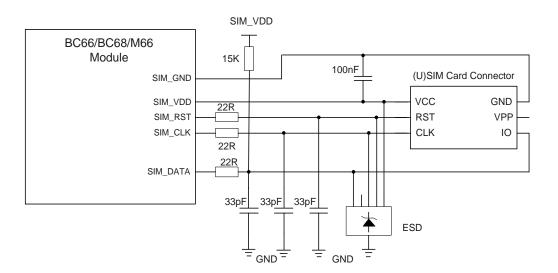
Figure 10: Reference Compatible Design for 6-Pin (U)SIM Interface
