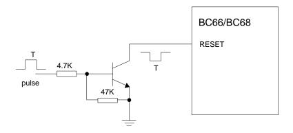
Figure 7: Reference Circuit of RESET by Using Driving Circuit
