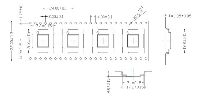
Figure 19: Tape Dimensions (Unit: mm)
