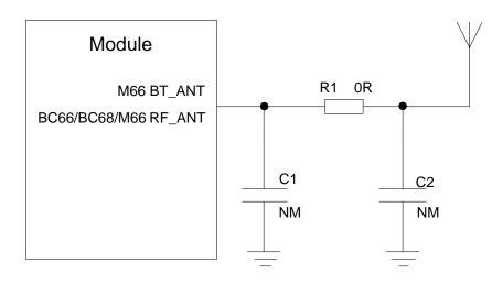
Figure 12: Reference Circuit of RF Antenna Interface
