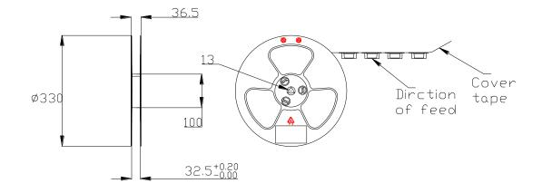
Figure 20: Reel Dimensions (Unit: mm)
