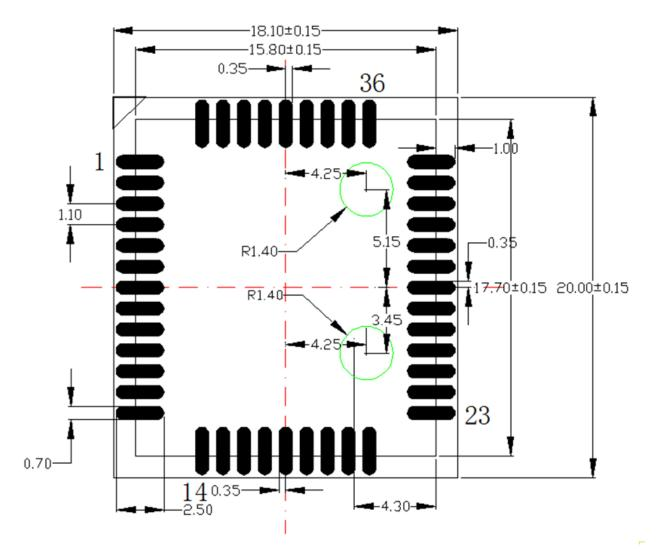
Figure 16: Recommended Stencil Design for M66 (Unit: mm)
