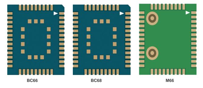
Figure 13: Bottom View of BC66/BC68/M66
