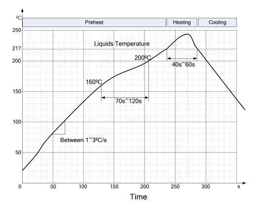
Figure 18: Reflow Soldering Thermal Profile
