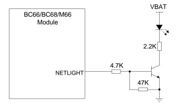
Figure 9: Reference Circuit of NETLIGHT
