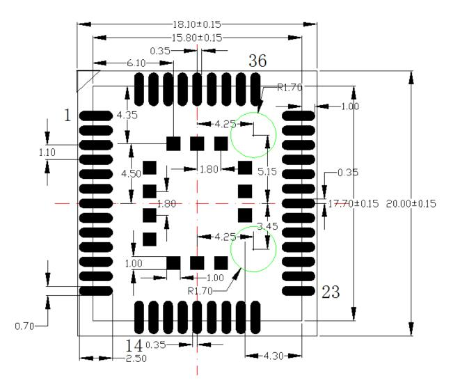
The following figure shows the recommended compatible footprint of BC66, BC68 and M66.
