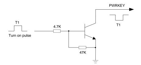
Figure 4: PWRKEY Driving Circuit for Module Turn-on (BC66/M66)
