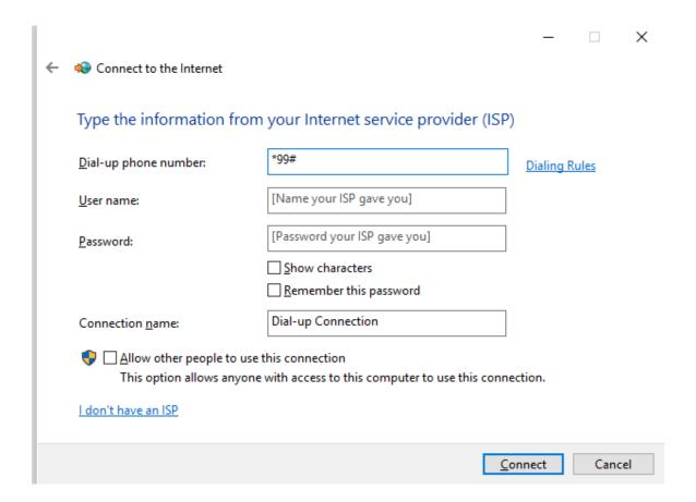
**Figure 12: Configure the Connection**
