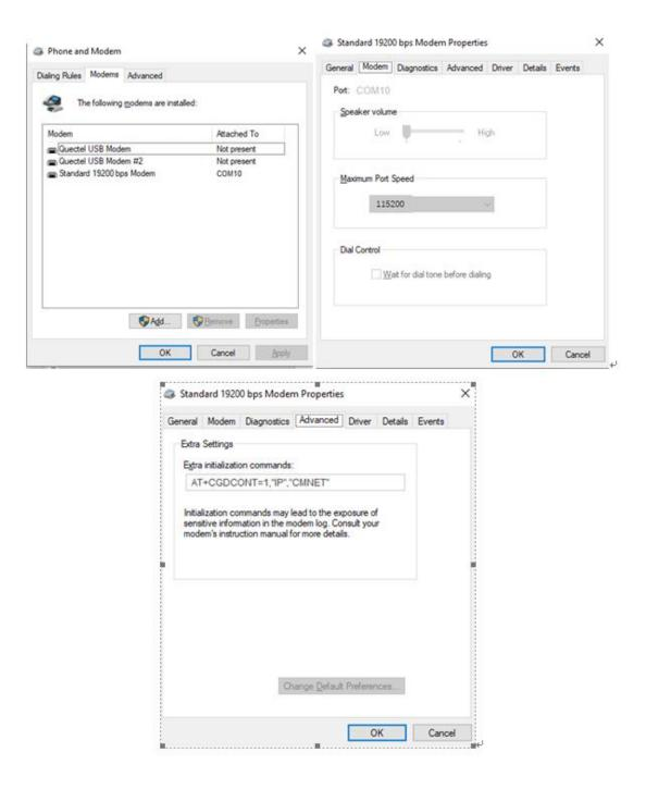
Figure 9: Configure the Modem Driver
