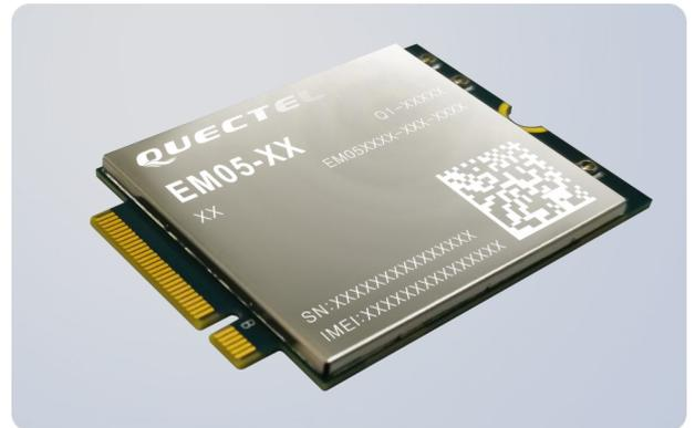
Quectel EM05 is an LTE category 4 module adopting standard M.2 (NGFF) form factor. The space-saving M.2 form factor allows EM05 to be easily integrated into smaller and thinner devices. With a maximum data rate of 150Mbps downlink and 50Mbps uplink, it is optimized specially for M2M and IoT applications.
