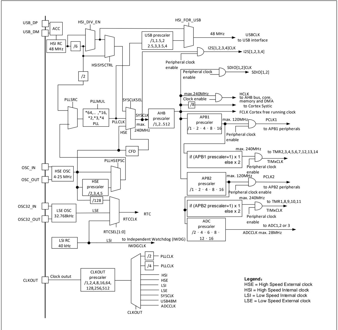
(1) When using USB function and its clock source is from PLL, CPU frequency must be 48 MHz, 72 MHz, 96 MHz, 120 MHz, 144 MHz, or 192 MHz; when its clock source is direct from HSI 48 MHz, CPU frequency can be any frequency from 48 MHz to 192 MHz.
