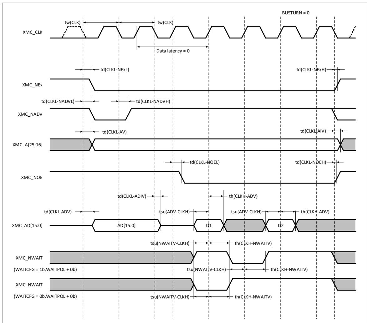
**Table 34. Synchronous multiplexed PSRAM/NOR read timings<sup>(1)(2)</sup>**
