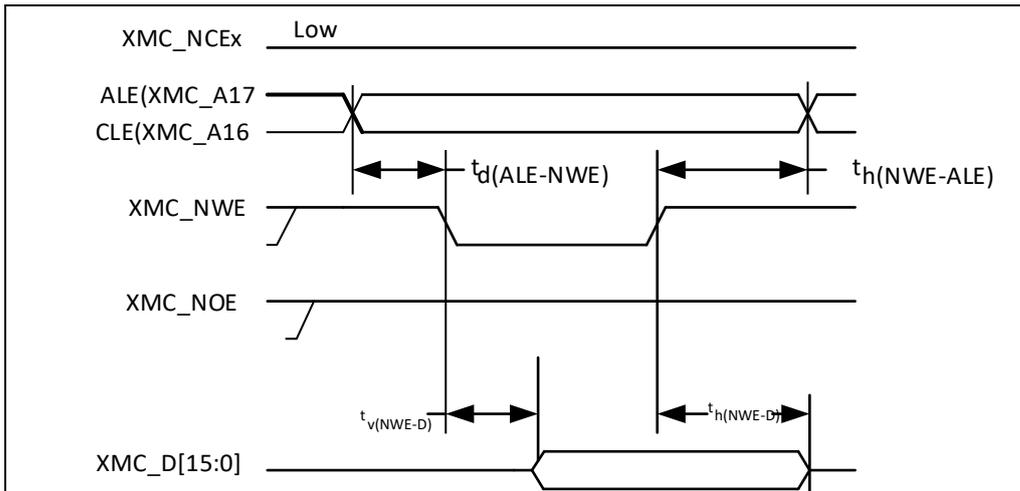
**Figure 27. NAND controller waveforms for common memory read access**
