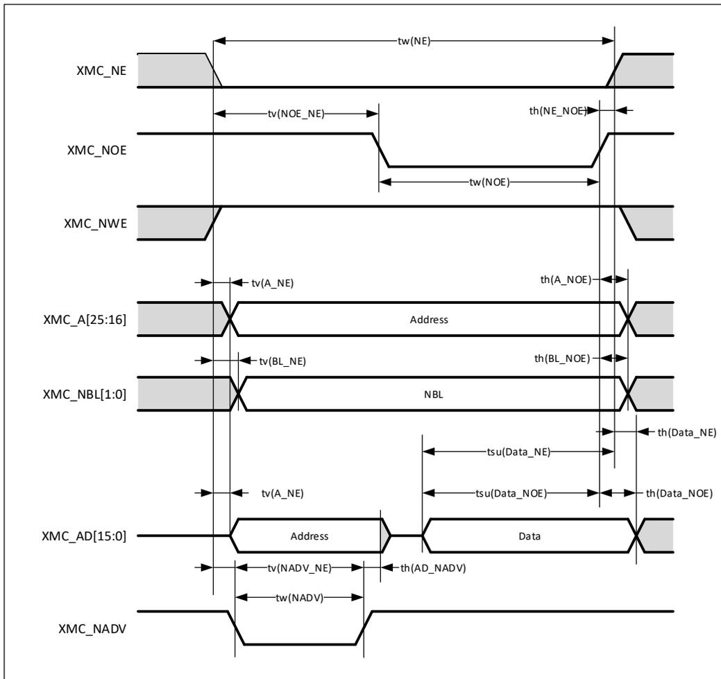
**Table 32. Asynchronous multiplexed PSRAM/NOR read timings<sup>(1)(2)</sup>**
