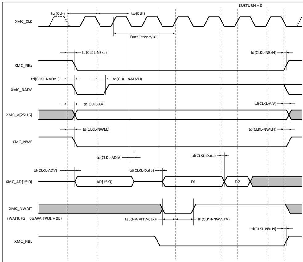
**Table 35. Synchronous multiplexed PSRAM write timings<sup>(1)(2)</sup>**
