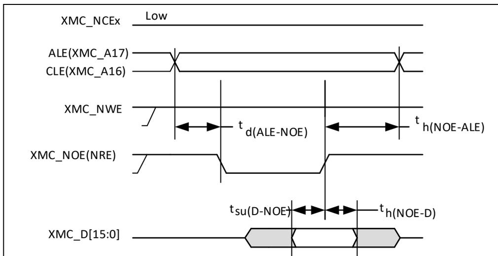
**Figure 26. NAND controller waveforms for write access**
