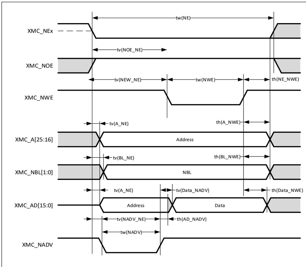
**Table 33. Asynchronous multiplexed PSRAM/NOR write timings<sup>(1)(2)</sup>**
