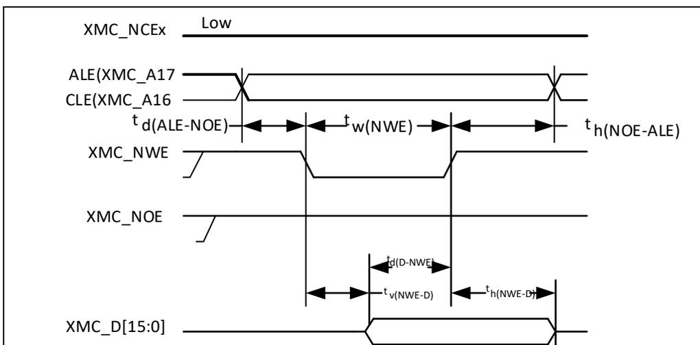
**Table 36. Switching characteristics for NAND Flash read and write cycles<sup>(1)</sup>**
