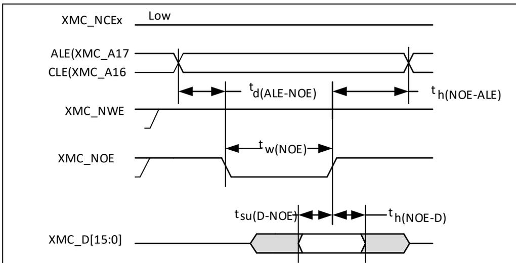
**Figure 28. NAND controller waveforms for common memory write access**
