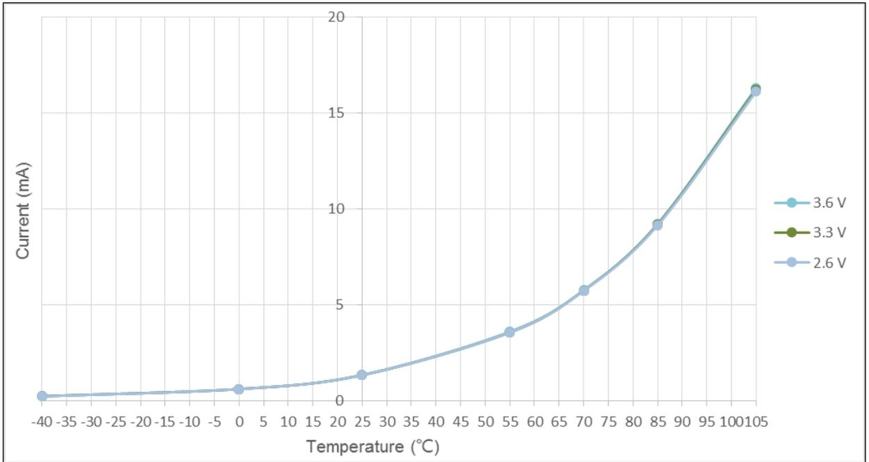
Figure 14. Typical current consumption in Standby mode vs. temperature at different V<sub>DD</sub>
