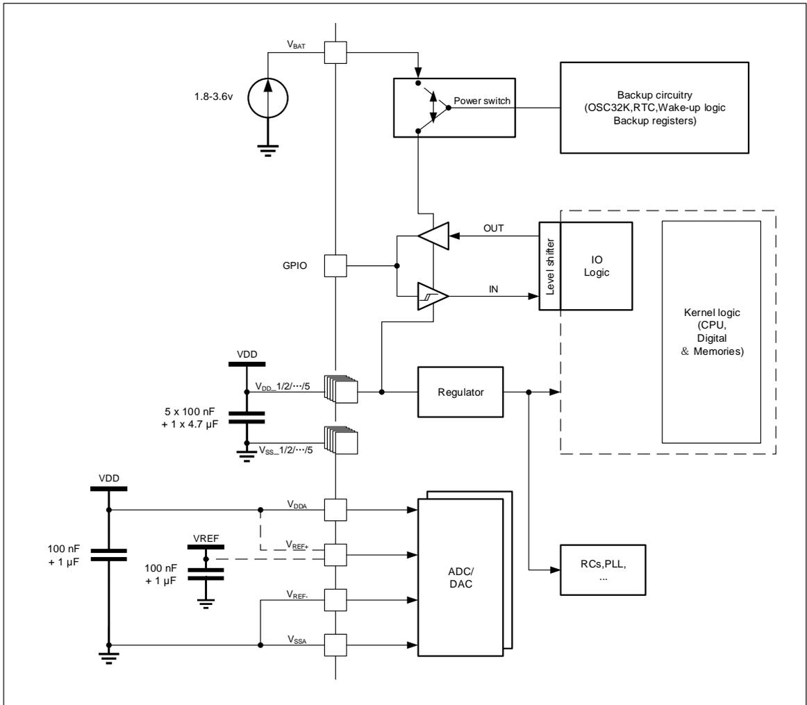
Caution: In this figure, the 4.7μF capacitor must be connected to V<sub>DD3</sub>.
